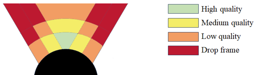
FIGURE 29: A POINT CLOUD'S QUALITY CATEGORY IS ASSIGNED BASED ON DISTANCE AND FOV
