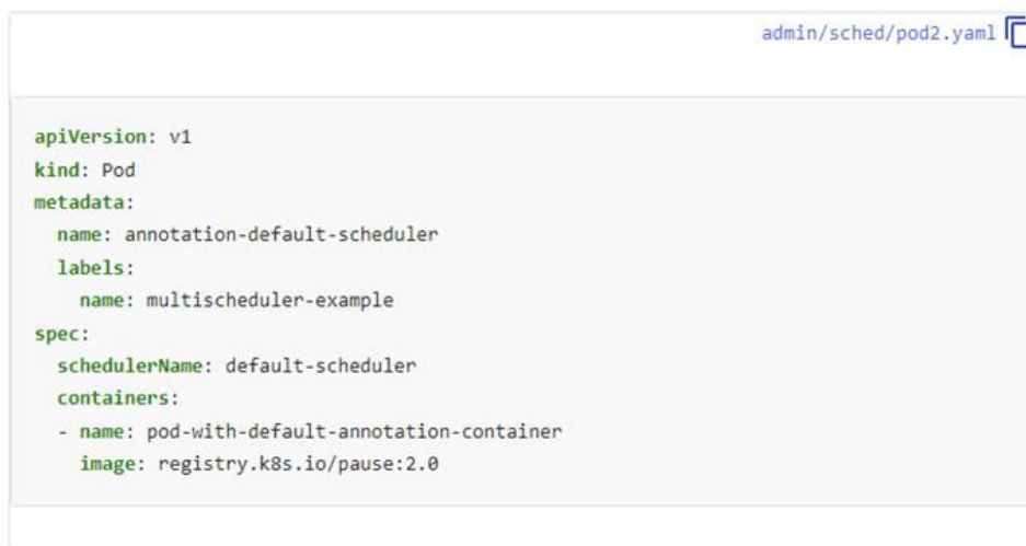
FIGURE 26: EXAMPLE THAT SPECIFIES A SCHEDULER FOR POD DEPLOYMENT
