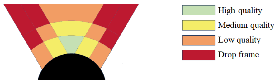
FIGURE 30: A POINT CLOUD'S QUALITY CATEGORY IS ASSIGNED BASED ON DISTANCE AND FOV
