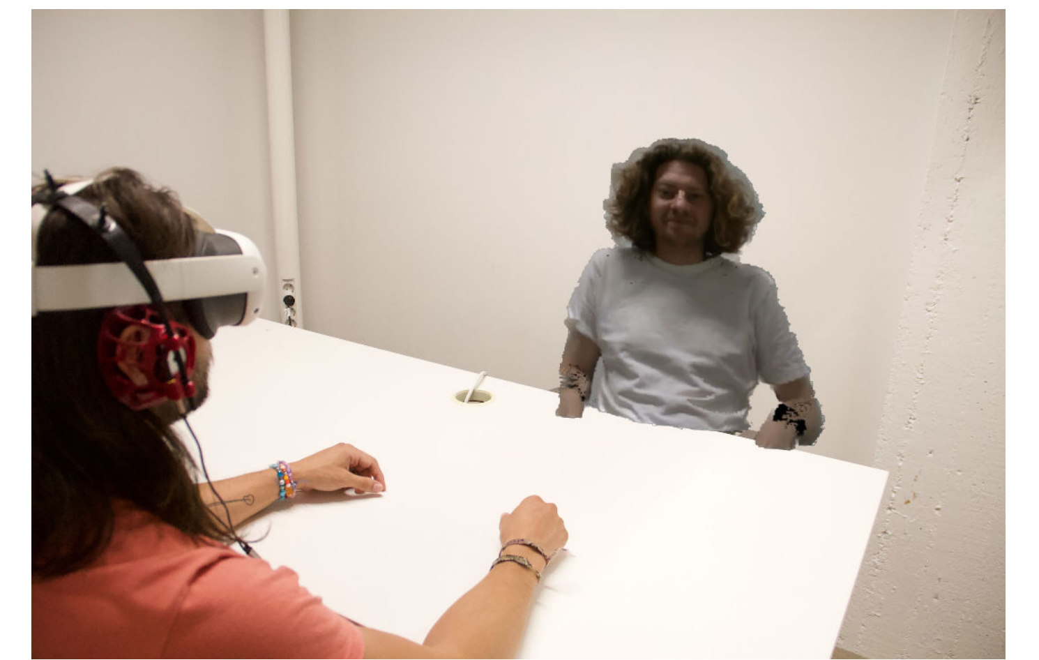
Fig. 4: Holographic calling setup with HMD + transparent headphones.
